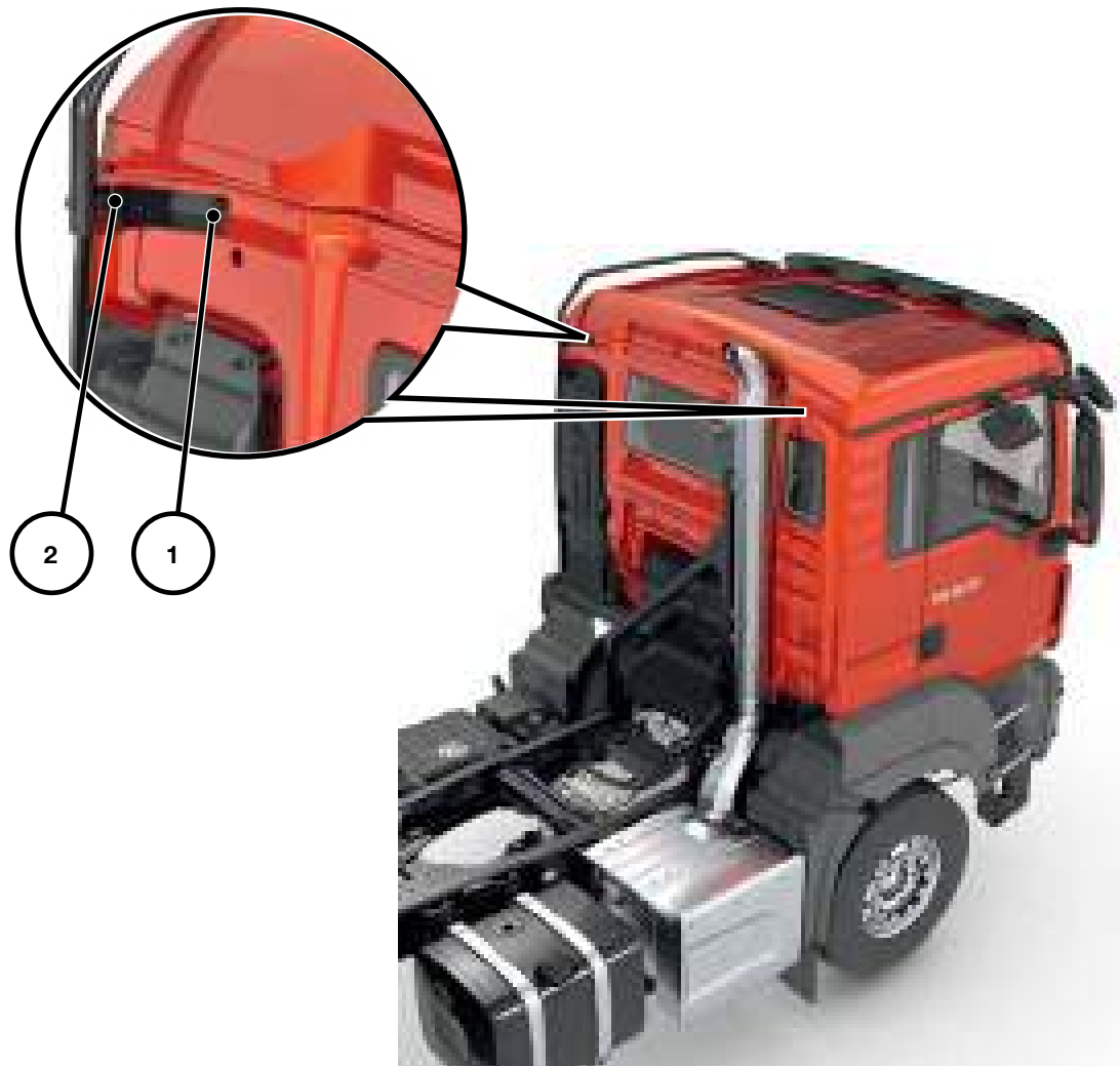
Fig. 30-III: Additional fastener for roofwalk
