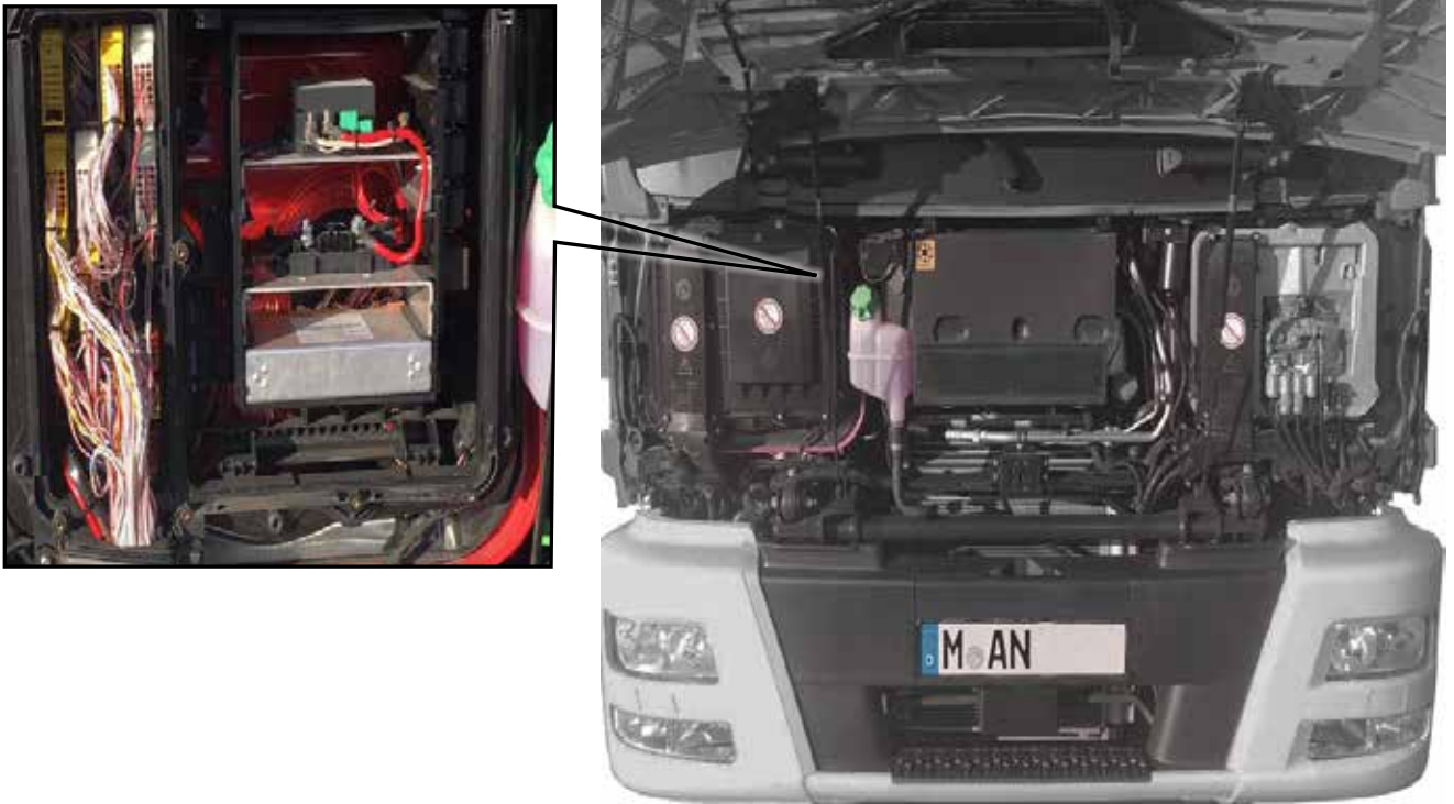
Fig. 112-III: Installation location of additional 50A body interface
