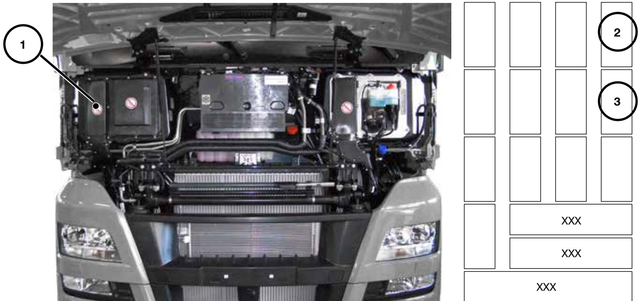
Fig. 104-III: Installation location of ISC interfaces
