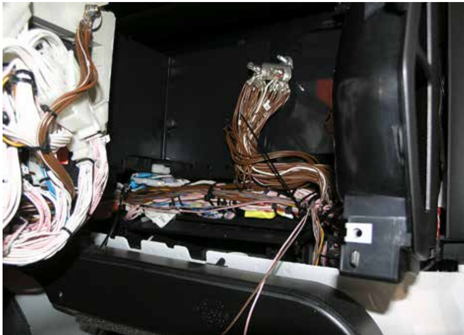
Fig. 114-III: Ground point X1644 behind central electric unit
