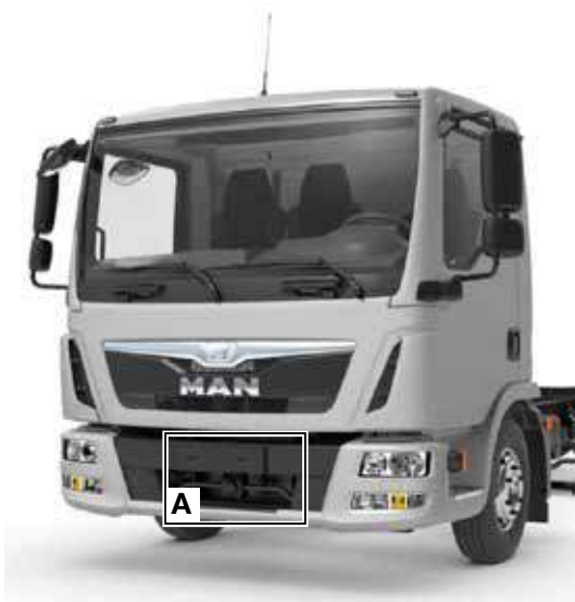
Fig. 118-III: Cab front showing installation location of radar sensor
