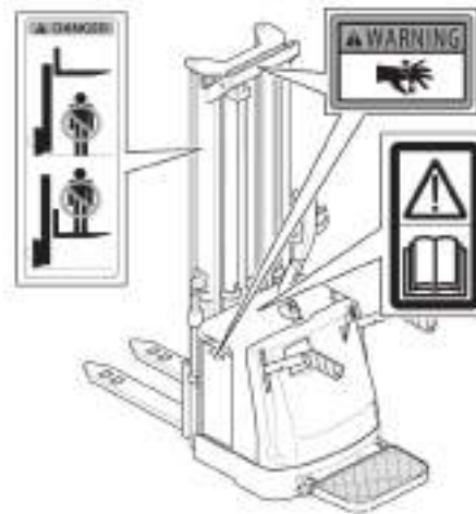
Locations of safety and warning signs on TS
