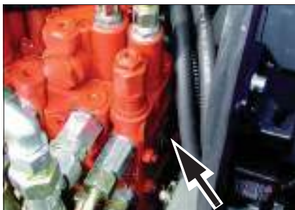
Fig. 6: Main valve block type label
