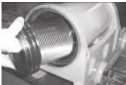
Fig. 48: Fitting the piston tube
