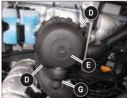
Fig. 20: Removing the housing section (from serial number AG03216)
