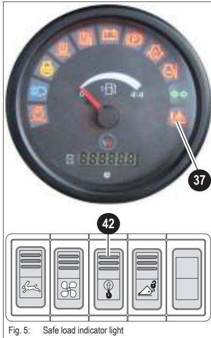
Fig. 5: Safe load indicator light
