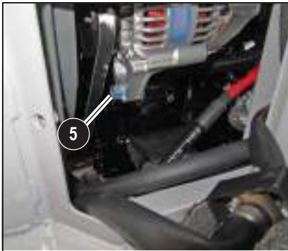
Fig. 33: Slackening the fastening screws
