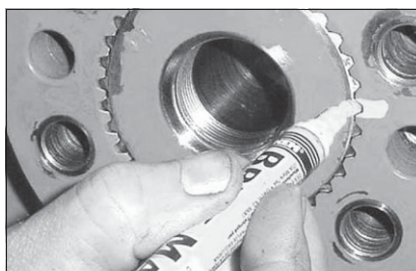
Fig. 60: Mark on shaft and securing ring
