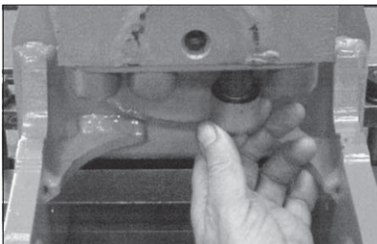
Fig. 75: Fastening the shaft screws
