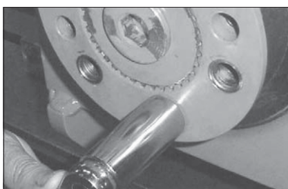
Fig. 65: Removing the bolts
