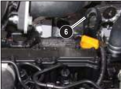
Fig. 34: Removing the shackle
