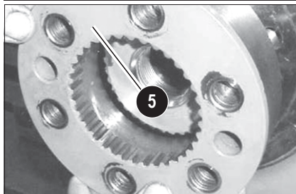
Fig. 59: Installing the securing ring
