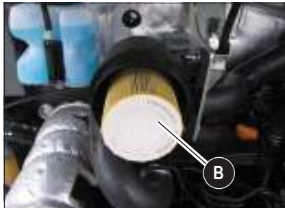
Fig. 21: Removing the outside air filter element
