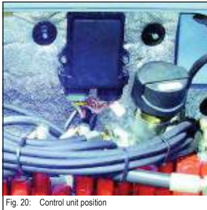
Fig. 20: Control unit position
