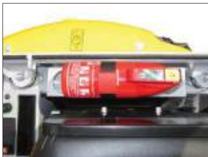
Fig. 92: Fire extinguisher in canopy
