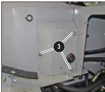
Fig. 31: Slackening the fastening screws
