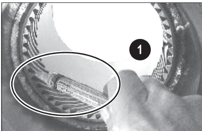
Fig. 30: Redrawing the dead centre mark of the ring gear
