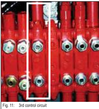
Fig. 11: 3rd control circuit
