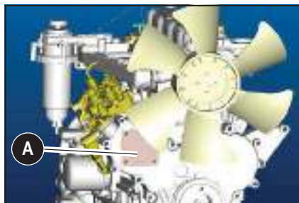
Fig. 13: Gear casing cover
