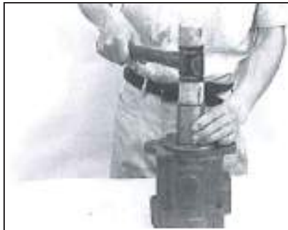
Fig. 15: Fitting the rotary shaft lip seal
