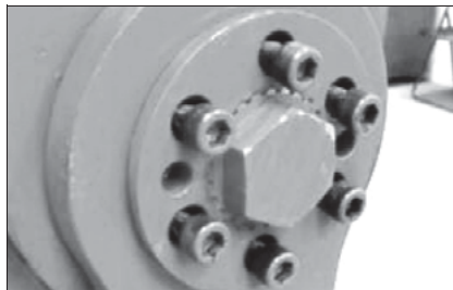
Fig. 83: Slackening the screws of the securing ring
