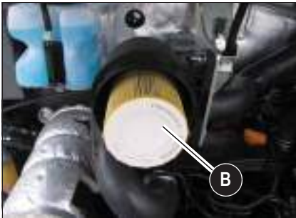
Fig. 24: Removing the outside air filter element
