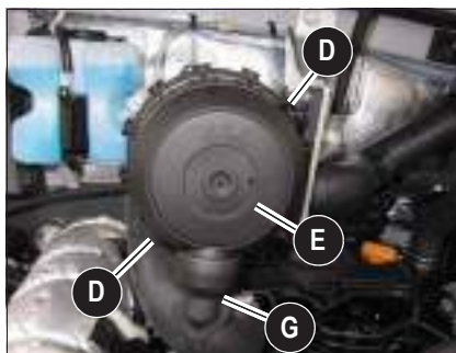
Fig. 23: Removing the housing section (from serial number AG03216)
