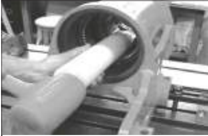
Fig. 21: Removing the piston tube with a hammer and drift
