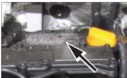
Fig. 4: Diesel engine number
